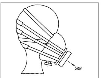
Figure 1 — Arrangement for testing connector
