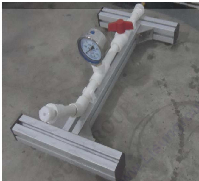
Figure 3: UL Sprinkler test device
