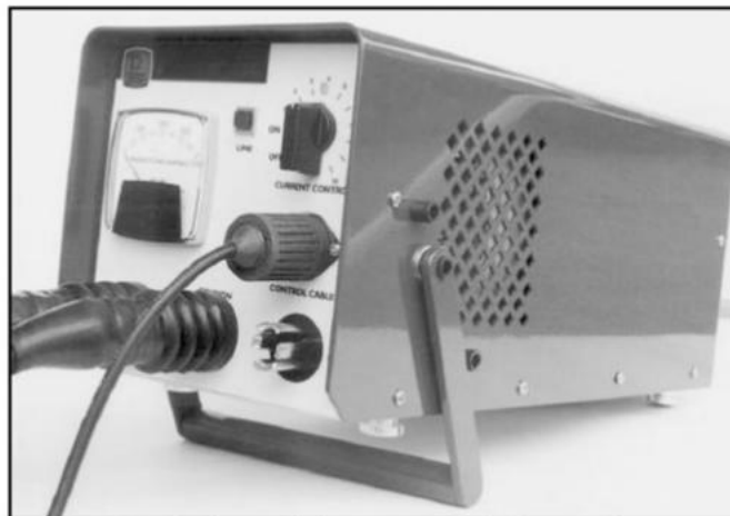
Typical portable power pack for prods
