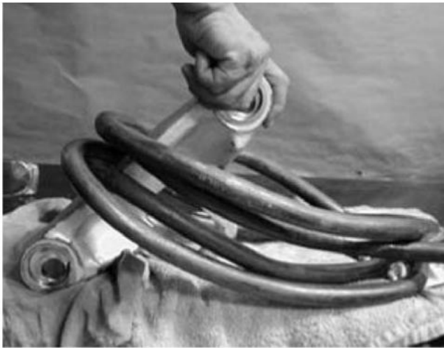
FIG. 9 Cable Wrap Magnetization
