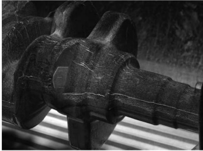
FIG. A1.4 Crankshaft with Various Longitudinal Indications
