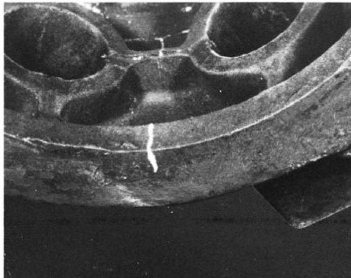
FIG. A1.19 Indication of Surface Cracks (Produced by Circular Indirect Magnetization, AC Continuous)
